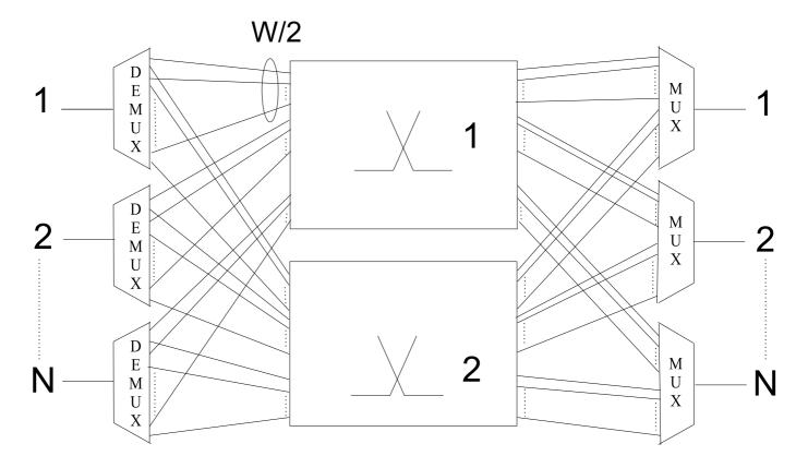
Fig. 10. Multi-plane node using structure (c).
