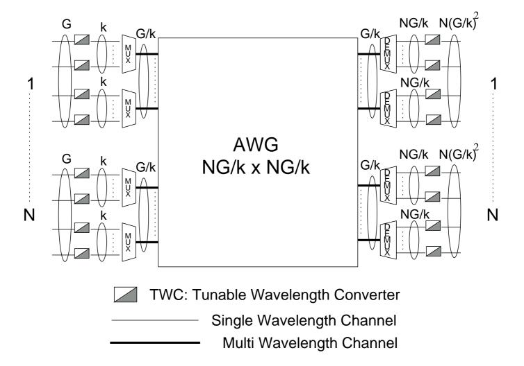
Fig. 8. Switching matrix with structure (b)
