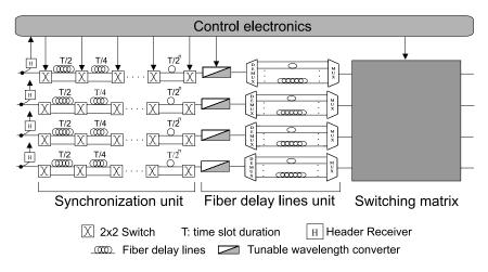
Figure 4. Detailed structure of one of the W/G parallel switching planes
