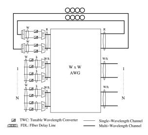
Figure 7. Optimized switching matrix
