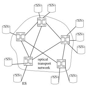
Figure 1. The optical transport network architecture
