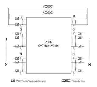
Figure 5. Basic switching matrix
