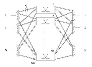
Figure 3. Optical packet-switching node general architecture
